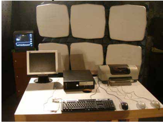
Figure 4.1.1. Generic Test set up for the Yeong Yang YY-7301 Personal Computer chassis
