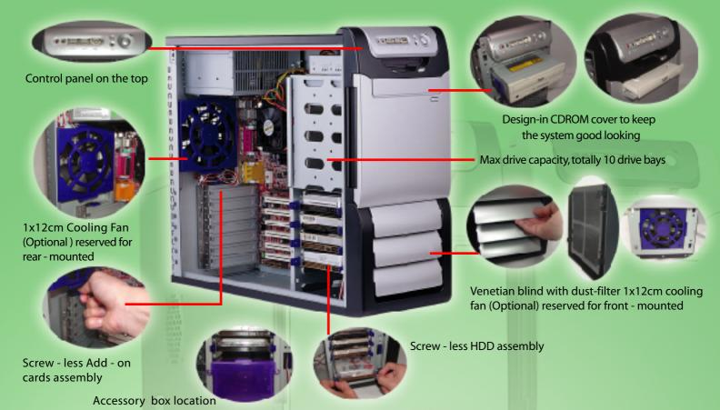
This is the illustration for structure of YY-5601 middle tower along with various front bezels
