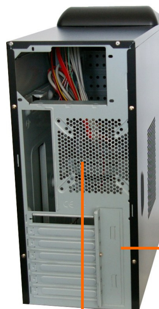
8,9 or 12cm fan for rear & 12cm for front-mounted
