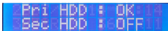
©Switch in Single mode (OFF indicates power for secondary drive is OFF)
