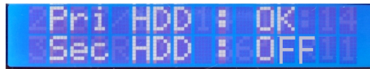
©Switch in Single mode (OFF indicates power for secondary drive is OFF)
