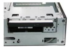
As EMI validated, the 3.5" hard drive will block the opening of chassis. No need to add shield cover.
