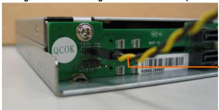
HDD Failure Signal Cable: 26H115311-001
