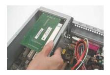
Slot the holder set into motherboard, and screw in the end of chassis.
