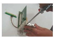
To slot in add-on cards into riser card and screw in bracket.
