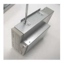
Install FDD & CD-Rom, mount driver bracket into chassis.
