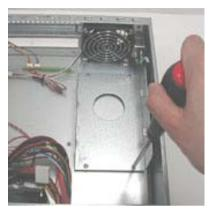
Remove the 3.5" HDD driver bracket.
